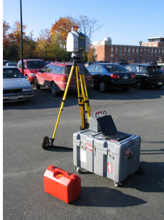
Figure 2.8: A typical scanning session with the Leica HDS3000
