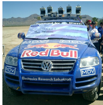
Figure 2.3: The winning vehicle of the DARPA Grand Challenge. Five LiDAR scanners are mounted across the top of the vehicle.
