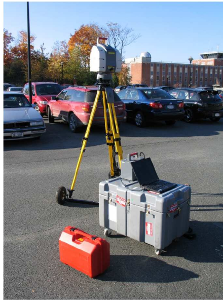
Figure 2.12: The setup of a typical scanning session with the Leica HDS3000. The scanner is mounted on a yellow tripod. The laptop and scanner battery are resting on the scanner's carrying case. The red box is a carrying case for the battery.
