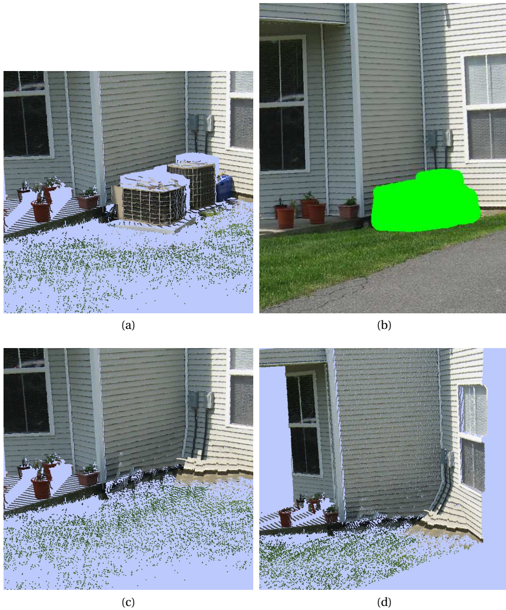
Figure 6.21: A data set for which we do not expect a good result. There is no information to guide the algorithm to fill the corner that results from the intersect of the two walls and the ground. (a) An image of the LiDAR scan. (b) The region to inpaint. (c) The holes appear to be filled correctly when hidden by the objects. (d) Visible artifacts are present in the resulting scene, including a warped corner and wall.
