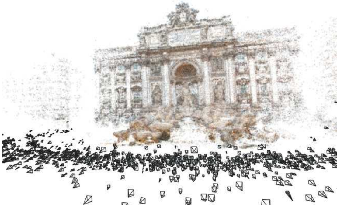
Figure 2.3: A 3D reconstruction of Trevi fountain from thousands of images. The locations of the cameras are shown as black pyramids. (Image from [11])
