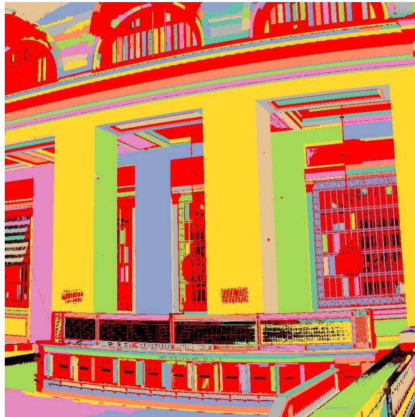
Figure 2.27: A planar surface LiDAR segmentation. Each surface is shown in a different color. (Image from [83])
