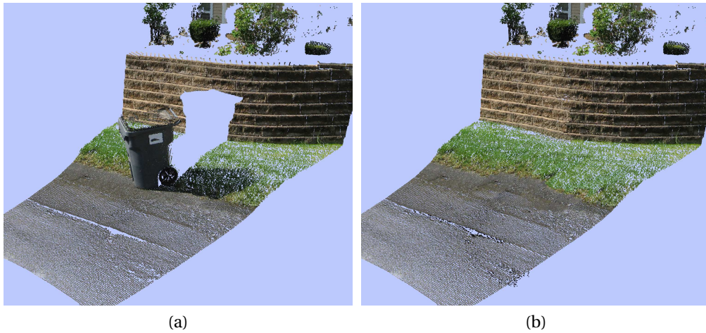
Figure 1.8: A visual summary of the work in Chapter 6. (a) A LiDAR scan with a large LiDAR shadow. (b) The inpainted LiDAR scan using our algorithm.
