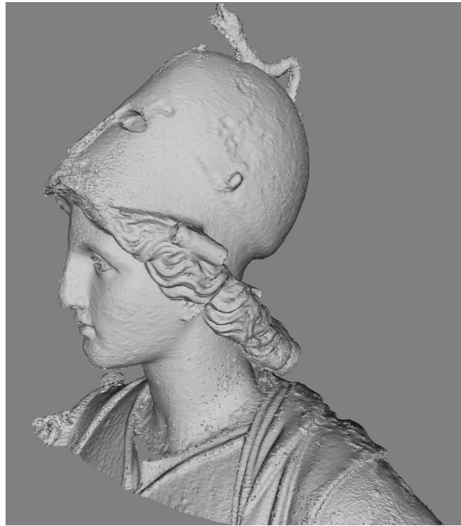
Figure 2.5: The resulting mesh after scanning a sculpture of a head with a structured light system. (Image from [13])
