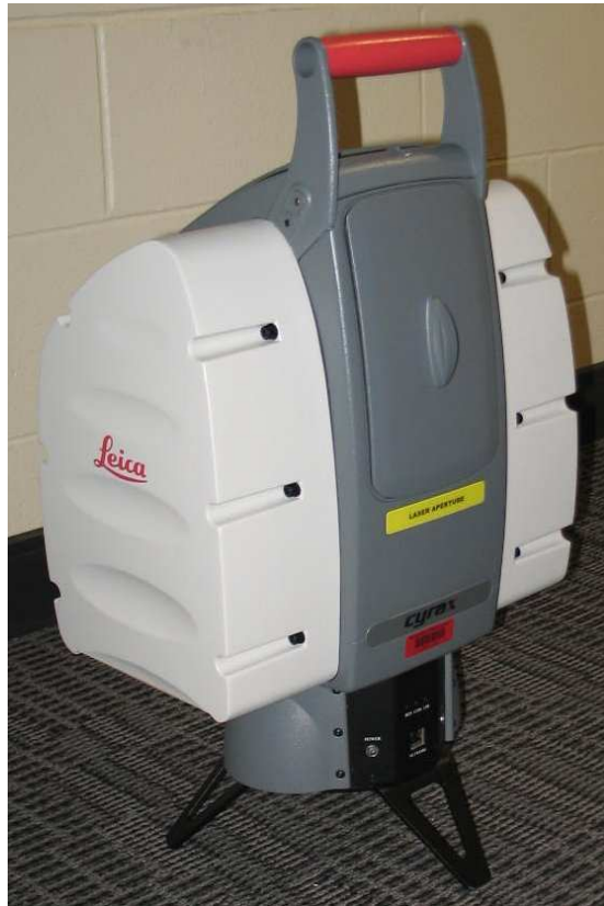
Figure 2.8: The Leica HDS3000 LiDAR scanner, used to acquire all of the data sets in this thesis.
