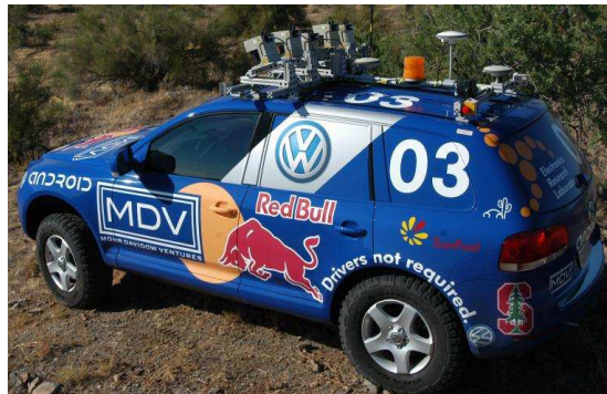
Figure 2.7: The winning vehicle of the DARPA Grand Challenge. Five LiDAR scanners are mounted across the top of the vehicle. (Image from [17])
