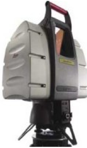
Figure 2.8: The Leica HDS3000 LiDAR scanner, used to acquire all of the data sets in this thesis.
