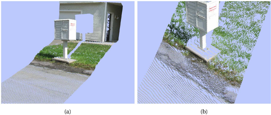
Figure 2.14: The glancing angle problem. (a) A scan of a mailbox and a building. (b) We see that the flat surface at the base of the mailbox was seen by a very small number of LiDAR rays compared to other surfaces in the scene.
