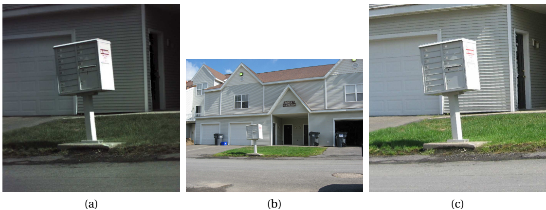
Figure 3.7: Recoloring the scanner image from a digital camera image. (a) The image from the scanner's internal camera. The image exposure is not ideal, and the image is of low quality. (b) The image acquired by an external digital camera. (c) The colors from the external camera mapped onto the scanner's image.
