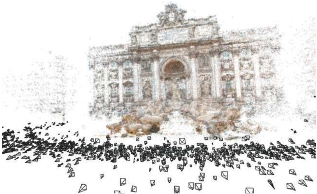
Figure 2.3: A 3D reconstruction of Trevi fountain from thousands of images. The locations of the cameras as shown as black pyramids. (Image from [4])
