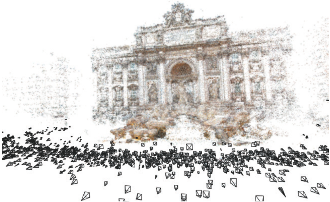
Figure 2.3: A 3D reconstruction of Trevi fountain from thousands of images. The locations of the cameras are shown as black pyramids. (Image from [4])
