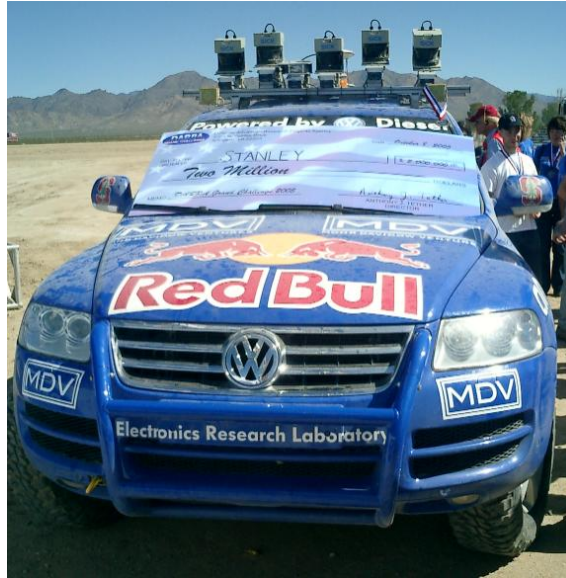
Figure 2.7: The winning vehicle of the DARPA Grand Challenge. Five LiDAR scanners are mounted across the top of the vehicle.
