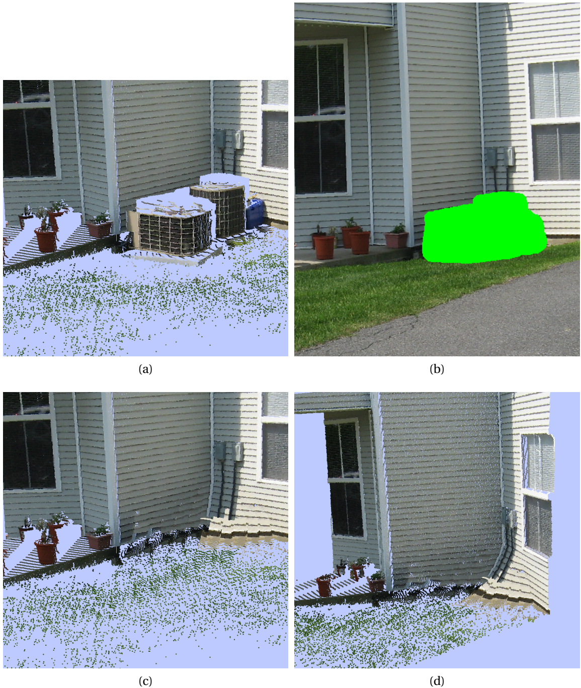
Figure 6.21: A data set for which we do not expect a good result. There is no information to guide the algorithm to fill the corner that results from the intersect of the two walls and the ground. (a) An image of the LiDAR scan. (b) The region to inpaint. (c) The holes appear to be filled correctly when hidden by the objects. (d) Visible artifacts are present in the resulting scene, including a warped corner and wall.
