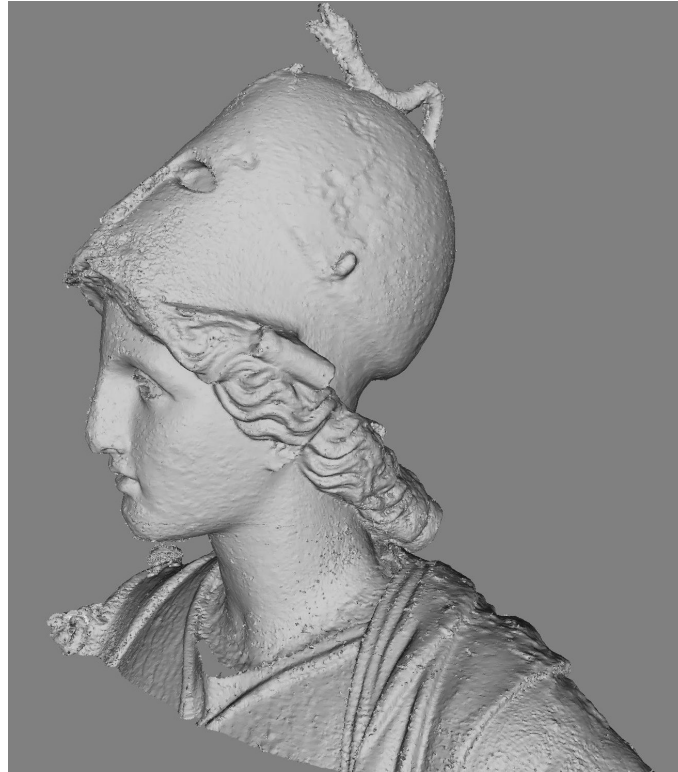
Figure 2.5: The resulting mesh after scanning a sculpture of a head with a structured light system. (Image from [129])
