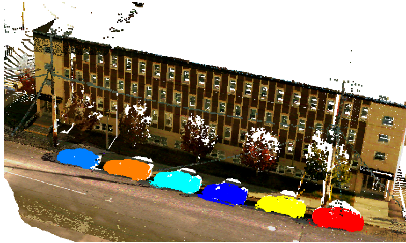
Figure 2.21: Several cars detected in a LiDAR scan. (image from [123])
