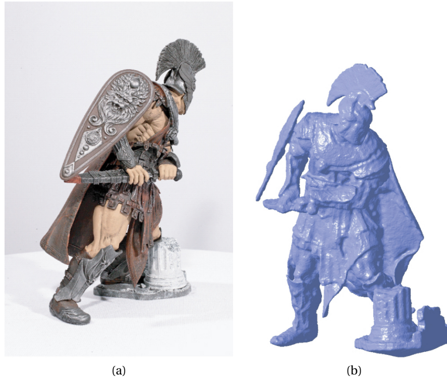
Figure 2.2: A 3D reconstruction of a soldier using the PMVS algorithm. (a) An image of a statue of a soldier. (b) A 3D reconstruction of the soldier from 48 images. (Images from [77])
