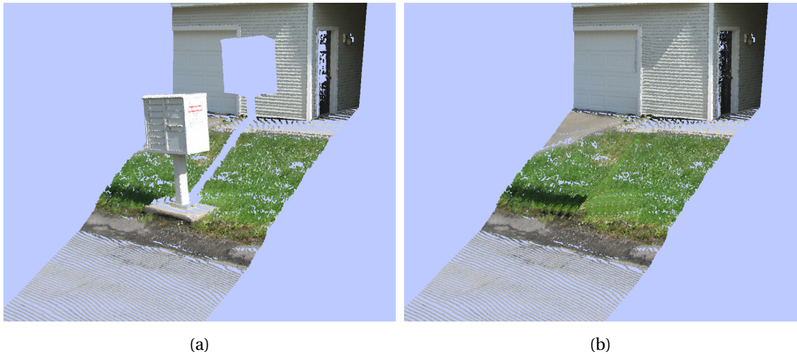
Figure 6.2: A demonstration of LiDAR inpainting. (a) A 3D scene of a mailbox with a building in the background. (b) The mailbox has been removed and the scene behind it has been filled using our proposed LiDAR inpainting algorithm.
