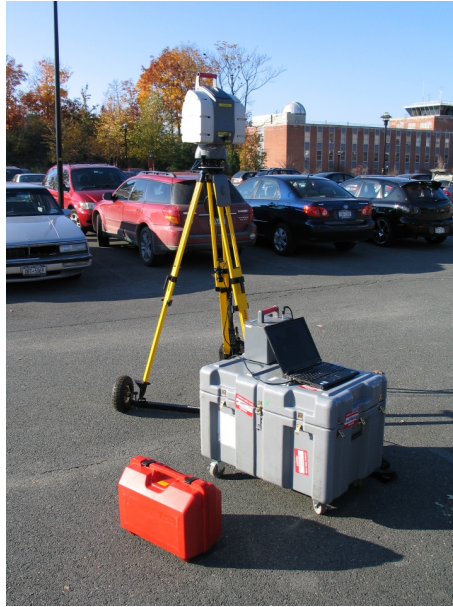
Figure 2.12: The setup of a typical scanning session with the Leica HDS3000.
