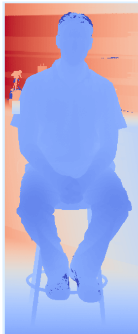
Figure 2.11: A depth image of a man sitting on a stool. Dark blue points are closest to the scanner, while dark red points are farthest from the scanner.
