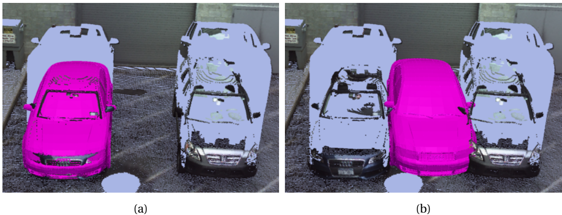
Figure 4.1: A motivating example of two detected object positions with similar scores, one of which is correct, and the other incorrect. (a) A car model correctly registered to the scene. (b) A car model incorrectly registered to the scene.
